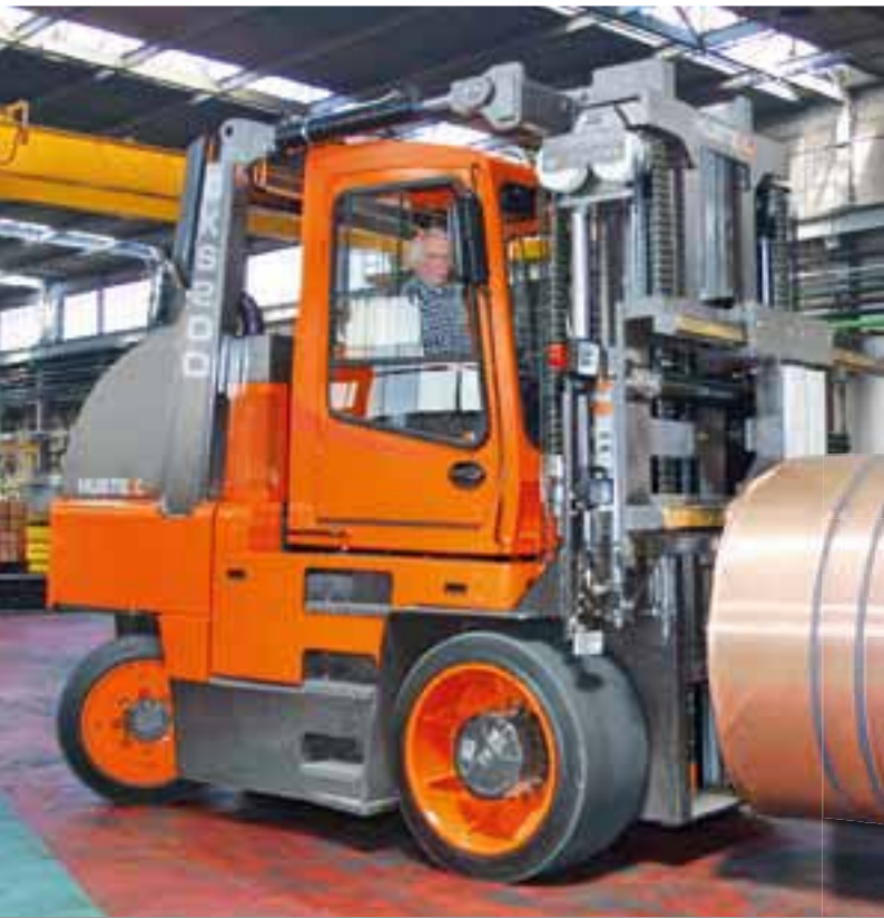
Gas-Kompaktstapler, Tragfähigkeit 20 t LPG-powered compact forklift, capacity 20 t
