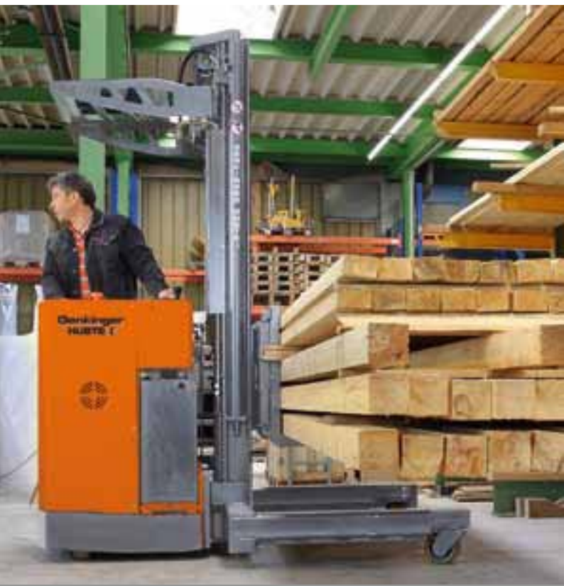
Elektro-Vierwege-Stand-Hochhubwagen Electric fourway high-lift truck with driver's stand
