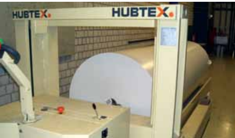
Deichselgeführter Papierrollen-Transporter Electric-powered pedestrian transporter for paper rolls
