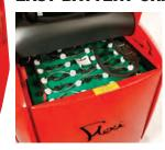
Low rear lift off or roll off for fast changeovers. Good access for battery topping. No motors hidden underneath.
