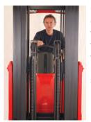
Operators have excellent forward visibility thanks to the triplex free lift mast, with its twin side mounted lift cylinders. Safe forward pallet pick up and set down.
