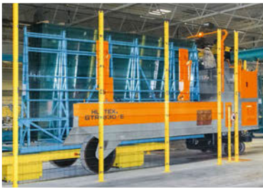
GTR 330 E unloading 33 tons stillage from cold end stacker
