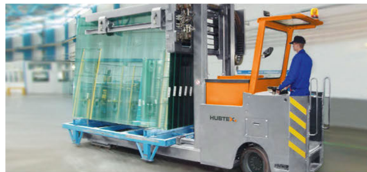
Glass securing device adjustable to different glass pack heights and widths
