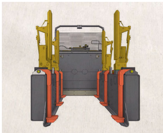
GTR with 180° foldable lifting arms to handle stillages with different widths
