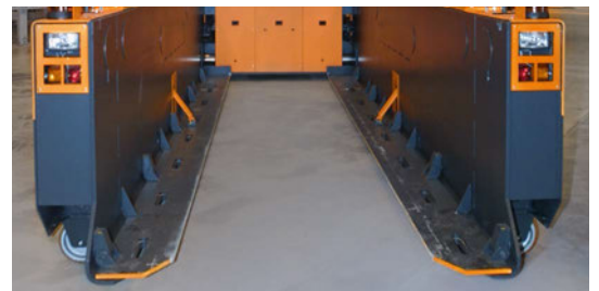
TR with adjustable loadarms to achieve
