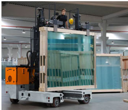
M 90 handling glass packs in end caps
