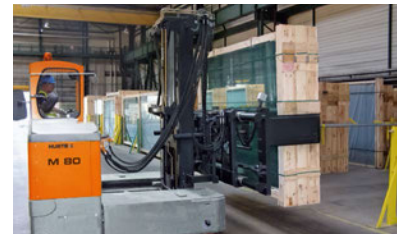
M 150 S0 stores glass packs in collars on two levels
