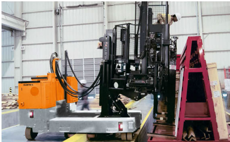
M 90 loading glass packs directly on a lorry
