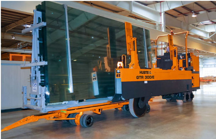
GTR unloading stillage from trolley
